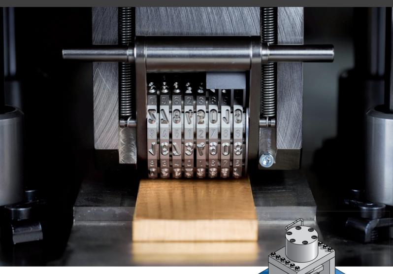
This system has been specifically designed to mark gold bars. The maximum pressure is 20 tons. So this system is able to press complicated engravings. The pressure is adjustable. For the consecutive numbering of the 1 Kg bar is included an automatically numbering head. The numbering head can be switched by hand or pneumatically. The press stroke is less than 5 mm. The press is equipped with a two-hand control.
