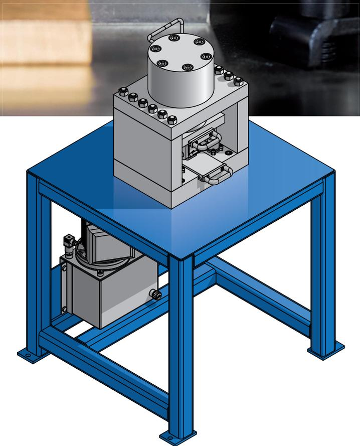
This system has been specifically designed to mark gold bars. The maximum pressure is 20 tons. So this system is able to press complicated engravings. The pressure is adjustable. For the consecutive numbering of the 1 kg bar is included an automatically numbering head. The numbering head can be switched by hand or pneumatically. The press stroke is less than 5 mm. The press is equipped with a two-hand control.
